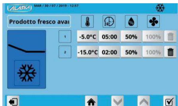
Advanced work cycle programming, with different sub-phases for temperature, humidity and fan speed
